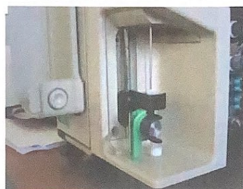
Intermediary position when moving between 'run' and 'flush'
